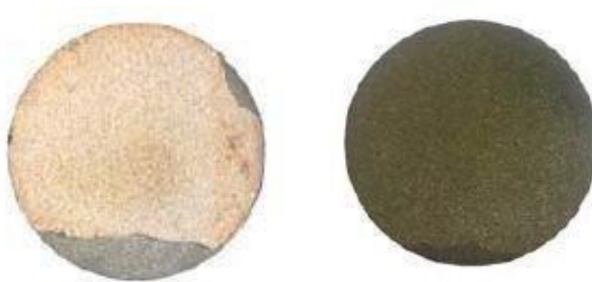
Fig.4. After Hot Corrosion (a) Mild Steel (b) Monel 400 Coated Material
